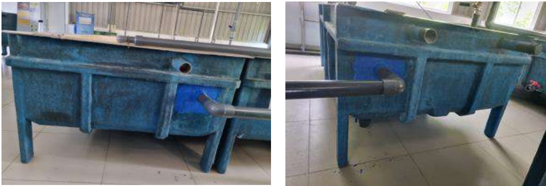
Figure 1. Re-circulating tank system after modification
